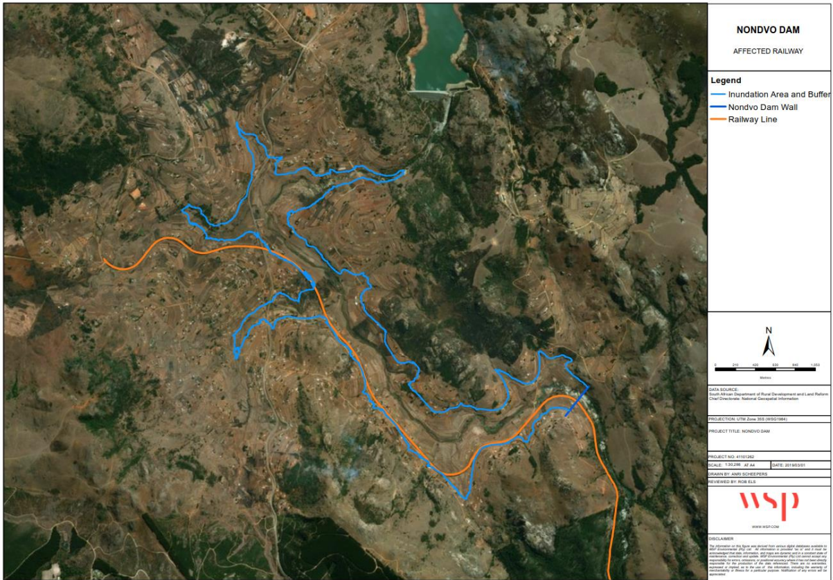
Figure 7-66: Existing Railway Line Route and Affected Section Requiring Relocation
