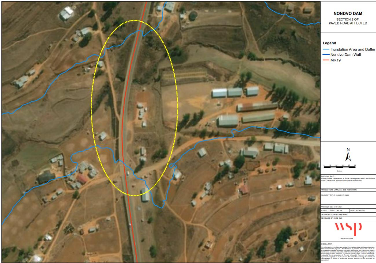
Figure 7-63: Section 2 of Paved Road Affected by the Proposed Reservoir
