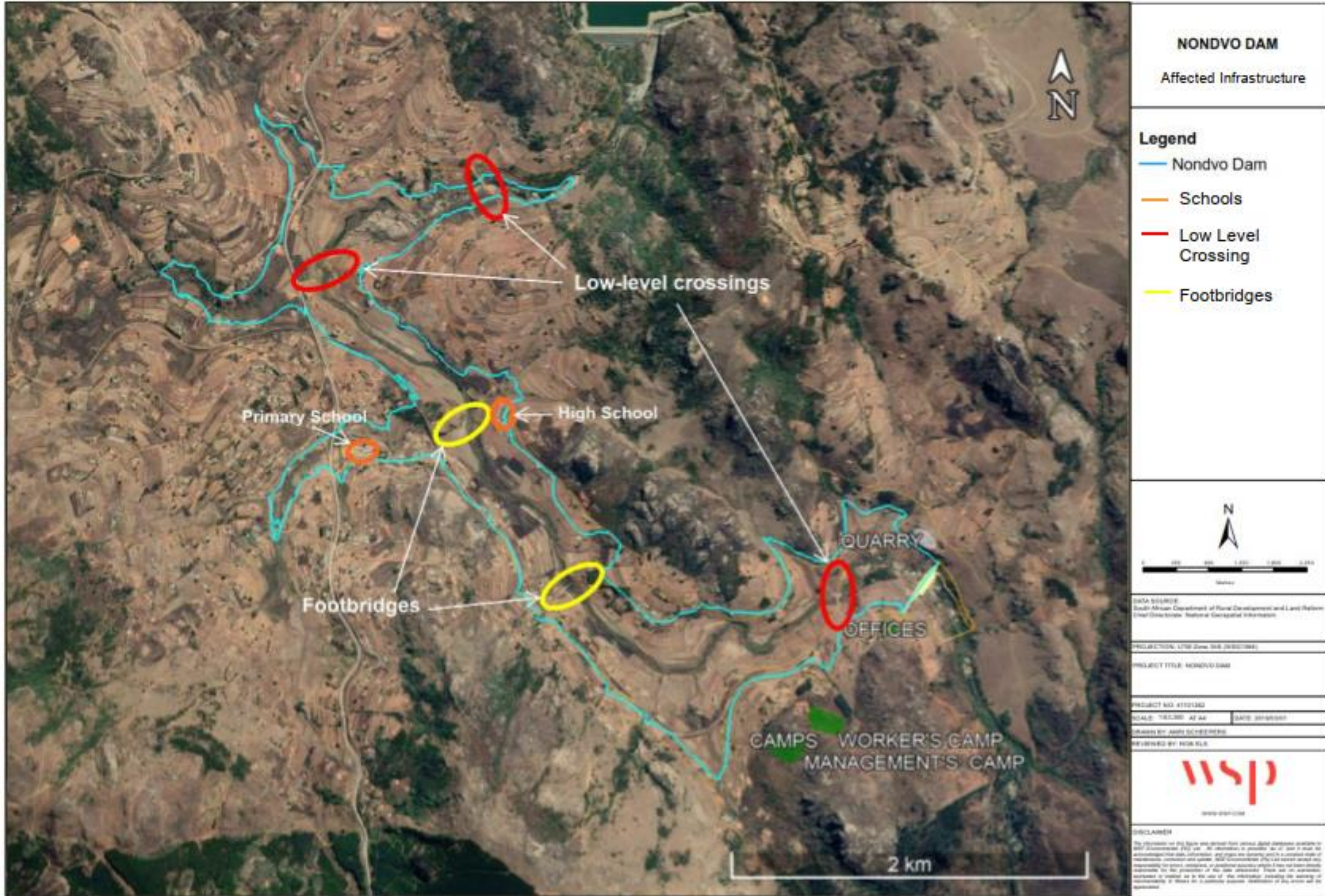
Figure Error! No text of specified style in document.-7: Layout showing the Project footprint including reservoir at flood level of 963.4 masl (blue line) and location of affected social infrastructure.
