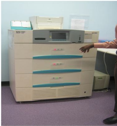
Figure 6: An MGit machine used to run samples for culture and DST at the National Reference Laboratory in Mbabane.
