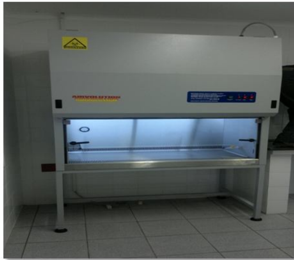
Figure 7: A Bio-safety cabinet installed at Mhlume RSSC laboratory in the Lubombo region. Used to run samples for culture and DST.
